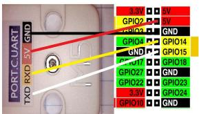
Unfortunately the supply lines (5V,GND) of the GPS unit must be crossed to match the pin assignment of the Raspi:
