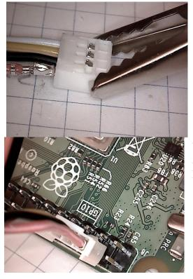
Then insert the two metal contacts (swapped over) back into the corresponding holes of the plastic plug. (see picture).
